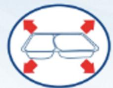
The aluminium dish must not come into contact with the walls of the microwave oven. (Minimum distance to the walls: 2cm.)
