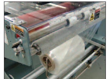
EZ Load Film Unwind and Adjustable Depth Pin Perforator with Brush Roller
